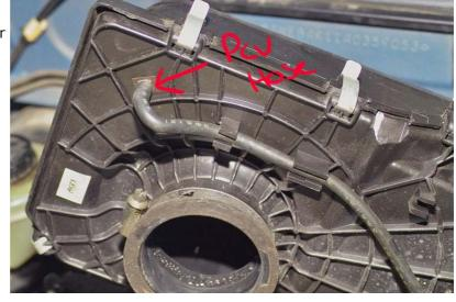
I currently don't know a better way to get off the old silicone other than hacking it to bits with a nice sharp new razor blade once a majority is removed I pried off the plate (need something very pointy, I just used the razor blade, first attempt I broke the blade then used the wider area caused by the break to pry it off. This revealed
