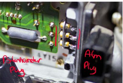
I reheated the two rows of three joints carefully (See Image on Left), wasn't sure which three need reheating.
