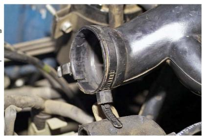
• You will find the airbox is firmly seated to the Throttle body. Pop your head down near the front of the motor (nearby the accessory belts) and look under the airbox there is a large hose clamp like device holding the air box firmly onto to the inlet of the Throttle Body, loosen this clamp. (See Image on the right).
